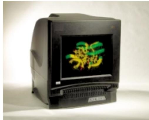
*The LightSpace DepthCube is the world's first solid-state volumetric 3D display. No headgear. No moving parts. Full color. 50 Hz refresh.*
