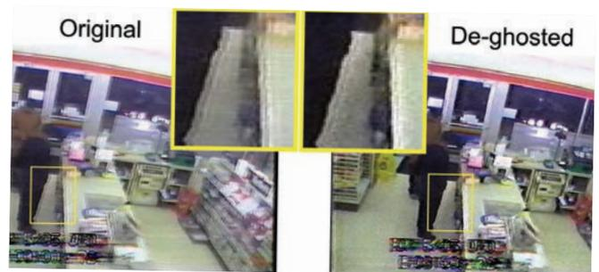
ABOVE Figure 1: To remove ghosts, computer science Ph.D. student Eric Rachlin estimated the spatial shift of the signals and the decay of the signal with each reflection.
