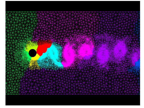
Fig. 2 Refined mesh at time t = 30 secs of incompressible fluid flow past a cylinder with Reynolds number Re = 250
