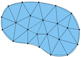
Fig. 1 Decomposition of a two-dimensional domain into a triangular mesh
