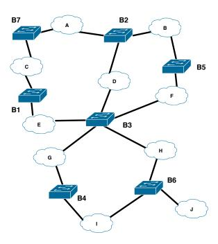
In the switched ethernet network above, which bridge ports will be disabled after the spanning tree algorithm finishes? Consider the bridges to be ordered B1, B2, ... B7.
