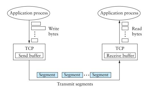
• Service model: "reliable, connection oriented, full duplex byte stream"
