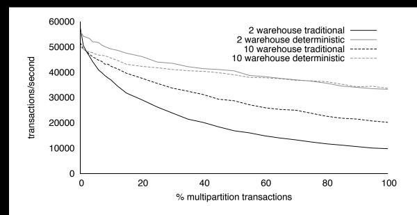
Figure 3: Deterministic vs. traditional throughput of TPC-C (100% New Order) workload, varying frequency of multipartition transactions.
