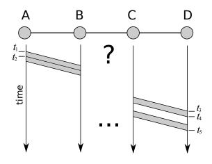
Setup: In the figure, assume there is no queueing or processing delay, and that nodes can forward a packet as soon as (a) *all* bytes for the packet have been received from the previous link, and (b) the outgoing link is free. All three links have a propagation delay of 10ms; link AB has a bandwidth of 10 Mbps ( $10^7$  bits per second), and link CD has a bandwidth of 8 Mbps ( $8 \times 10^6$  bps). You send two probe packets of 1000 bytes each, as depicted in the figure.
