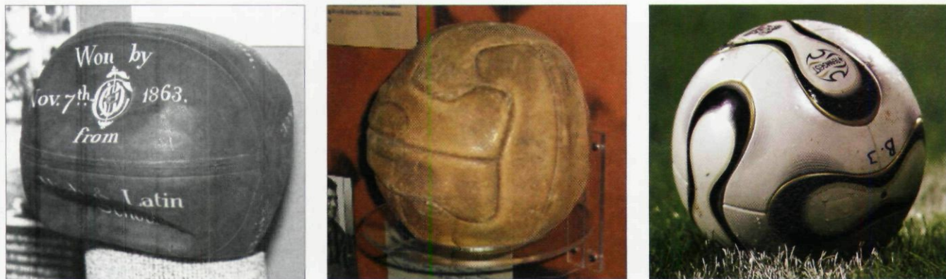
Figure 2. Soccer-ball design over the years has been driven by the demand for a round ball that holds its shape and by the technology available. Eight panels of vulcanized rubber were glued together to create the ball at left, used in the earliest soccer championship in the United States in 1863. The leather ball at center, used in the 1950 World Cup, has a design typical of its era. The small number of large, irregularly shaped flat pieces adversely affected its roundness. Thanks to improvements in materials and manufacturing, curved pieces in more complicated shapes can now be used. This year's World Cup ball (right) is made from 14 synthetic-leather panels cut in intricately curved shapes. In graph-theory terms, this ball is a truncated octahedron. (Historic photographs courtesy of Jack Huckel, National Soccer Hall of Fame; right photograph courtesy of firosporfoto.de.)
