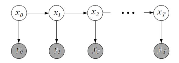
Measurement:  $y_t = Cx_t + v_t$   $v_t \sim N(0, R)$  Same as,  $p(y_{t+1} | x_{t+1}) = N(y_{t+1} | Cx_{t+1}, R)$ This is known as the Linear Gaussian assumption.
