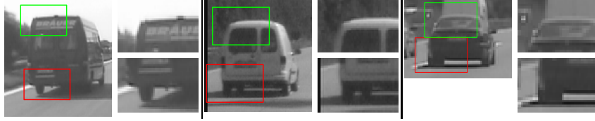
Fig. 1. Variation in the vehicle class of objects is shown. While objects shown here have a drastically different appearance as a whole due to the varying height and type of the vehicle, their components tend to be very homogeneous and are easy to model.
