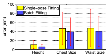
Fig. 8. Quantitative evaluation of shape. Accuracy of estimated body measurements (height, waist, chest) relative to ground truth. Batch estimation across pose decreases the errors.
