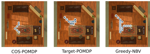
Fig. 4: Visualization of robot trajectory produced by different methods for the example shown in Fig. 3. A gray circle combined with a black line segment indicates a viewpoint.
