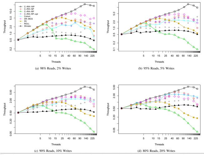
**Figure 6.** RWBench scalability results of various RW locks for varying read/write distributions: 2%, 5%, 10%, and 20% of write mode lock acquisitions. All graphs are in loglog scale. Here RCSLen = 4, WCSLen = 4, and NCSLen = 32. We vary the number of threads from 1 to 255 on the X-axis. Y-axis throughput is expressed in terms of aggregate million loop iterations performed per second.
