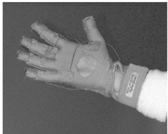
Figure 6. The Flex and Pinch input system. Although a CyberGlove™ is shown, any bend-sensing glove can be used.
