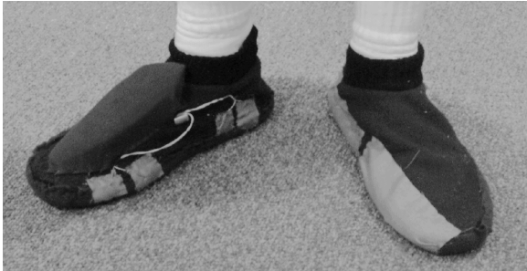
Figure 4. The Interaction Slippers allow users to tap either their toes or heels to invoke operations.
