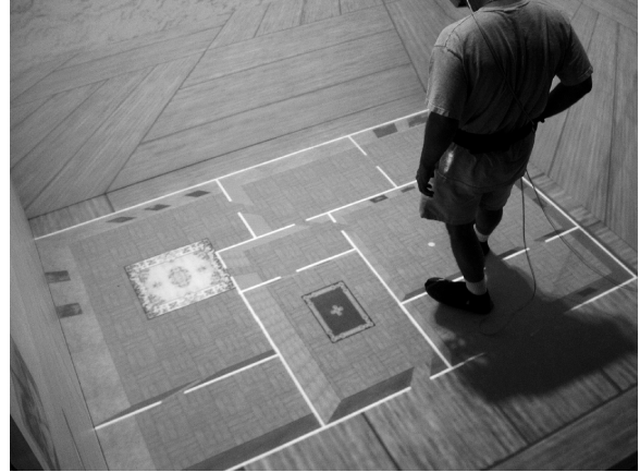
Figure 5. The Step WIM widget allows users to quickly navigate anywhere in the virtual world. The small sphere by the user's foot indicates his position in the miniature.
