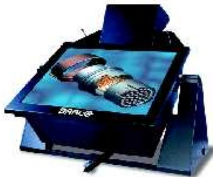
Figure 5.2: A Barco Baron rear-projected display device.
