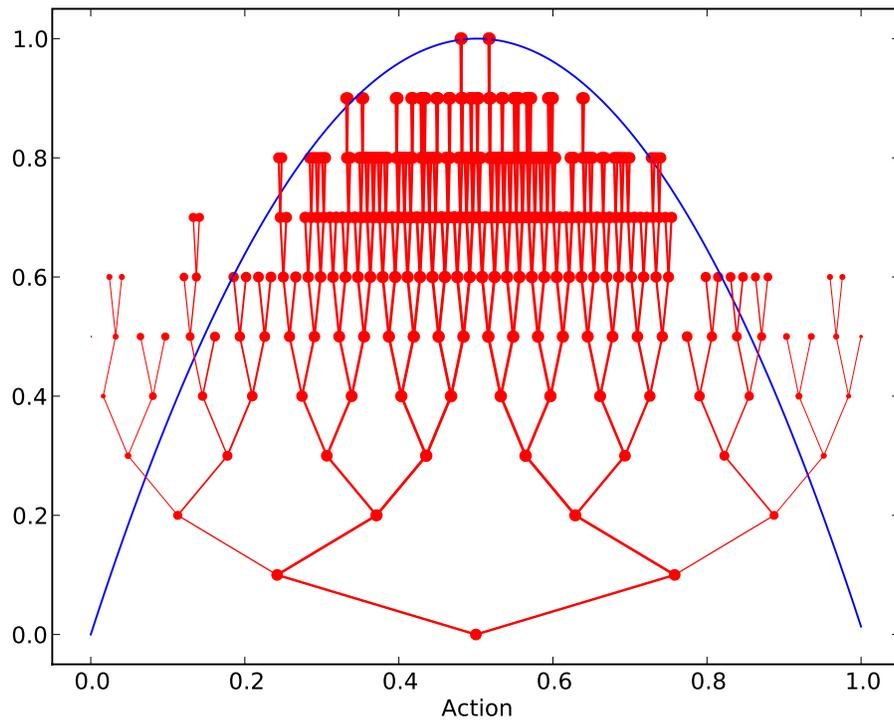
Figure 3.1: Illustration of the the tree built by HOO (red) in response to a particular continuous bandit (mean in blue). Thickness of edges indicates the estimated mean reward for the region each node covers. Note that samples are most dense (indicated by a deeper tree) near the maximum.
