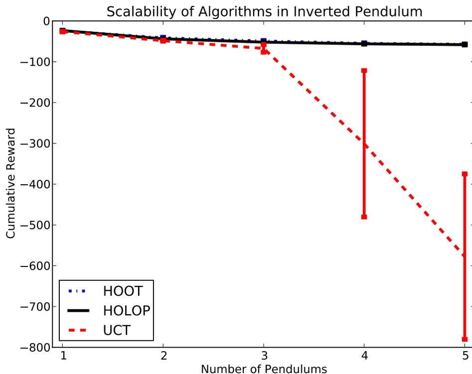
Figure 4.7: Performance of UCT, HOOT, and HOLOP while controlling multiple instances of the inverted pendulum problem.
