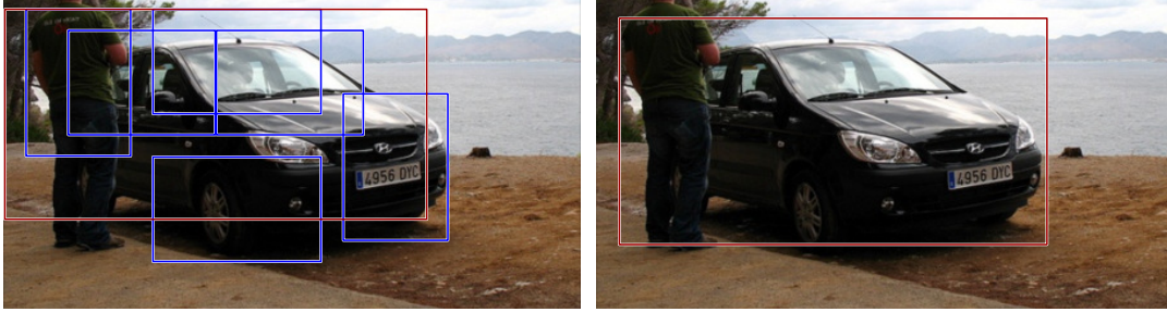
Figure A.1: A car detection and the bounding box predicted from the object configuration.
