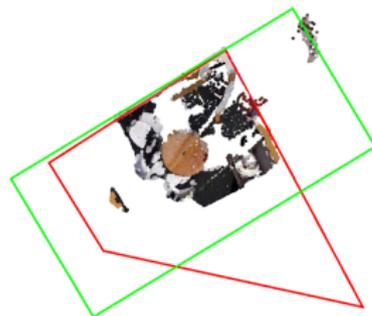
Sensor errors can mislead simple layout prediction heuristics (Song et al., 2015)
