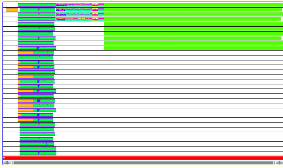
Figure 3. The Transaction-Task Visualization. Each row of the visualization corresponds to a user thread. Colors indicate the transaction and task the thread is working on. Time is represented along the X-axis.
