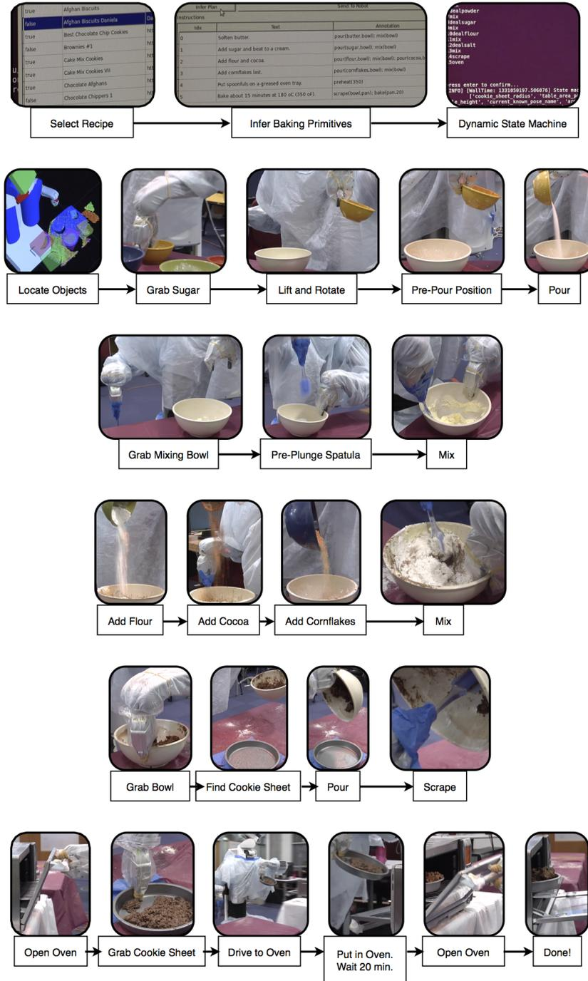
Fig. 5 A pictorial timeline of the baking process.
