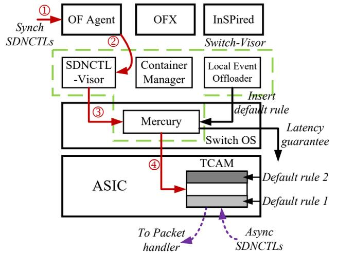
Figure 3: Switch Architecture
