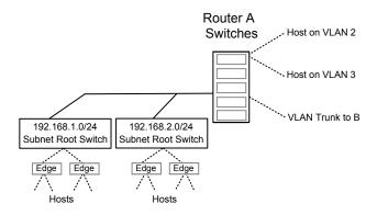
Figure 4: Exodus prototyping subnets and hosts adjacent to router A (other routers not shown). Every non-VLAN subnet is assigned a root switch, and every root has an edge switch per attached router. VLAN access ports are assigned one host each.
