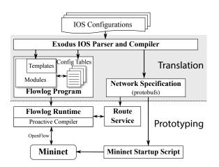
Figure 1: Workflow: Exodus produces Flowlog libraries and a network specification, which can be prototyped in Mininet [19].
