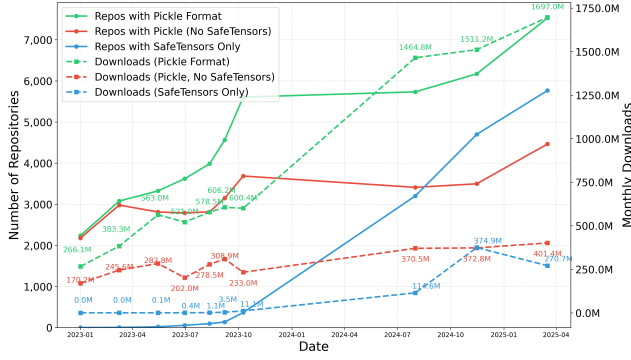
Figure 2: A longitudinal analysis of Hugging Face model formats for repositories with \geq 1000 monthly downloads. Repositories can contain multiple models, each in different formats. Each color groups repositories by the model formats they contain: at least one pickle model (green), exclusively pickle (red), and exclusively SafeTensors (blue).
