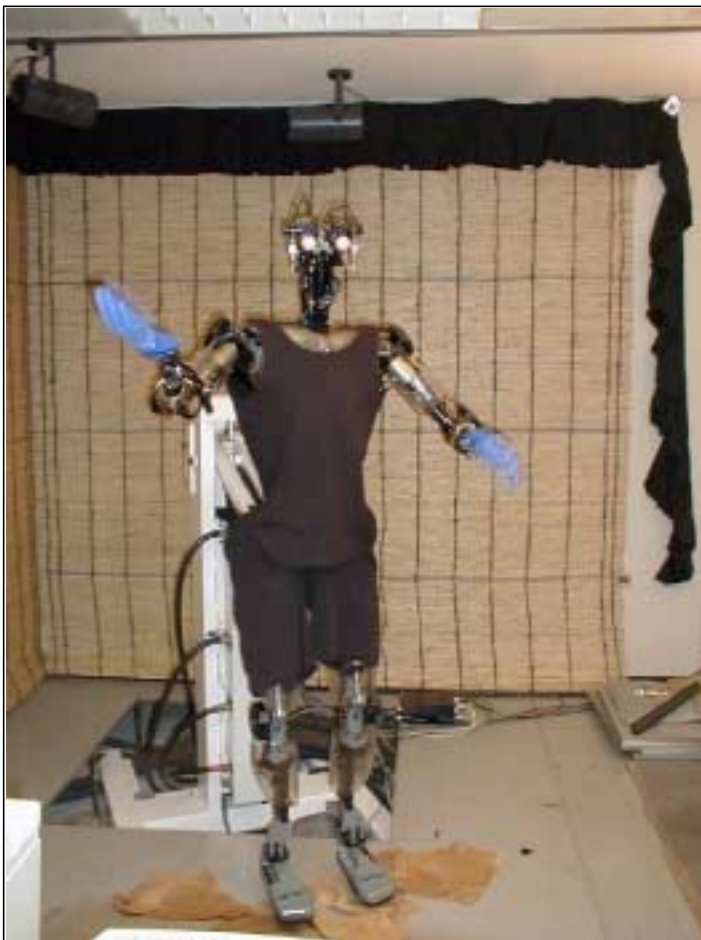
The humanoid robot DB in action. The paper towels under his feet are to soak up leaking hydraulic fluid!
