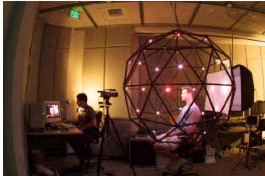
Andy sitting in an early version of Lightstage 3.0 with only 41 light sources and a simple static matting system using a single camera. The control program running on the PC is operated by Jonathan Cohen '00
