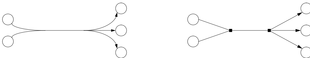
Figure 6-5: Approximation of a hyperedge (left) in the GELO presentation (right). The edge body and each of its branches is represented as a simple edge, and the edge’s source and destination junctions are represented as GELO nodes.
