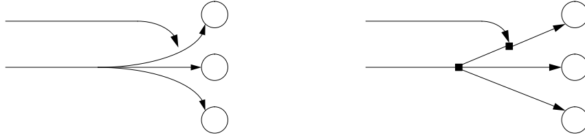
Figure 6-6: Possible approximation of an edge terminating at another edge (left) by GELO (right). The SPG branch containing the input port is represented by a two simple edges and a GELO node.
