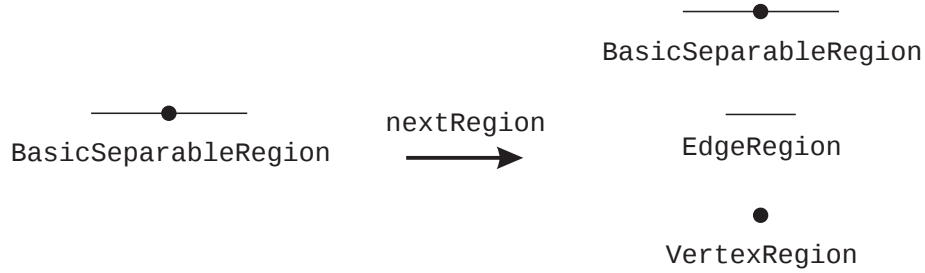
Figure 18: The possible objects returned by method nextRegion(Separator,Point2D,Discriminator) when invoked by a BasicSeparableRegion modeling a recursive decomposition of a horizontal subchain.
