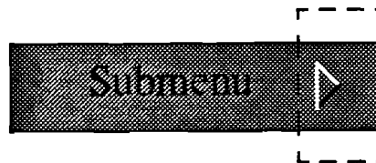
Submenu Button - The vertical dotted line indicates the region where the mouse needs to be in order to activate the submenu.
