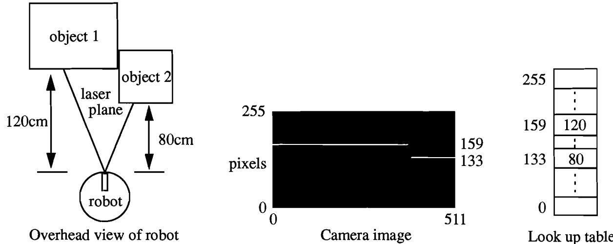
Figure 1: Calculating distances with the laser light striper.
