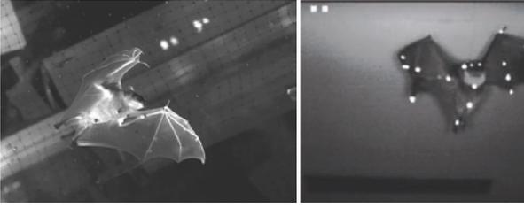
Fig. 1. Frames from wind tunnel videos recorded by high-speed digital cameras. Left: *Cynopterus brachyotis*, used in FastAero simulations. Right: *Pteropus Poliocephalus*, used in NekTar simulations. The 3D coordinates of markers attached to the bat wings are reconstructed using Direct Linear Transformation.
