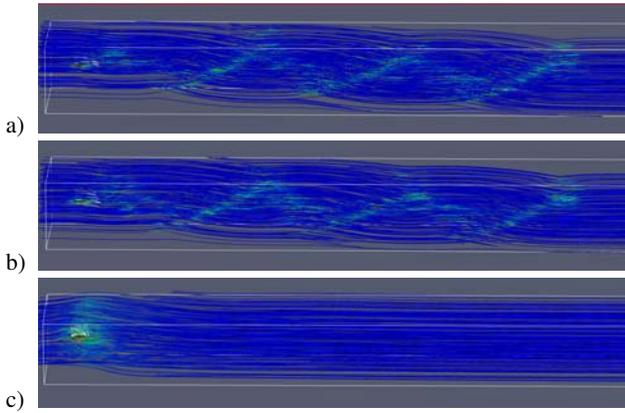
Fig. 4. Beginning of a downstroke. a) and b)  $v_{BFR}$  streamtubes in FastAero (curved and sharp wing), and c) in NekTar, colored by vorticity magnitude  $|\tilde{\omega}|$ .
