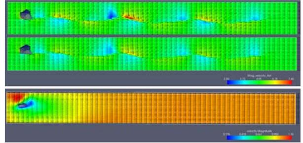
Fig. 7. Overview of  $v_{BFR}$  vectors and contours in FastAero (curved and sharp geometry) and NekTar. Color maps are different between the two cases; cutting plane is located at mid-body. Viscous effects are clearly manifested in the NekTar case.
