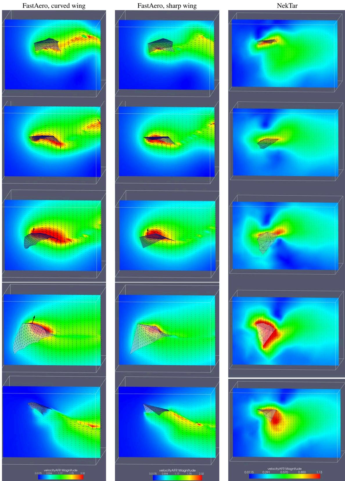
Fig. 10.  $v_{AFR}$ , FastAero and NekTar: Absolute velocity field in the mid-wing spanwise slicing plane during downstroke and upstroke. Viscous effects in NekTar are reflected in the behavior of the high  $v_{AFR}$  magnitude region, as the disturbance is manifested close to the wing surface. In FastAero, on the other hand, these regions are continuously shed from the wing.
