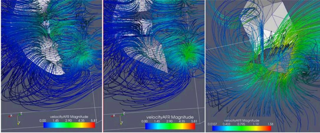
Fig. 6.  $v_{AFR}$  streamtubes in 3 cases (curved FastAero, sharp FastAero, and NekTar) in mid-downstroke. In both FastAero cases the streamtubes illustrate the effects of wing bound circulation and wake vorticity at leading and trailing edges.
