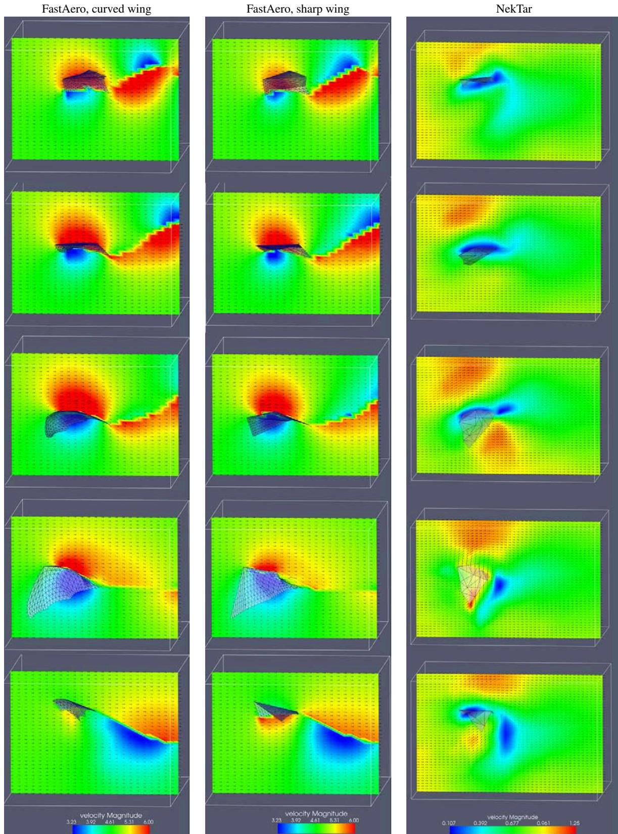
Fig. 9.  $v_{BFR}$ , FastAero and NekTar: Absolute velocity field in a spanwise slicing plane during downstroke and upstroke. In NekTar, the viscous effects force the flow to go slower at the surface of the wing, but this behavior is not seen in the FastAero cases. Since  $Re$  of the NekTar simulation is very low, the viscous effects are strongly manifested in the appearance of wide boundary layers.
