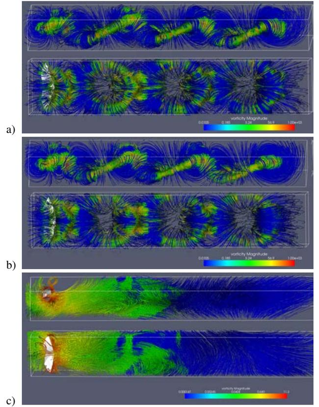
Fig. 5. Beginning of a downstroke. a) and b)  $v_{AFR}$  streamtubes in FastAero (curved and sharp wing), and c) in NekTar, colored by  $\log|\tilde{\omega}|$ .
