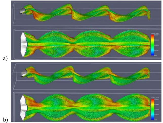
Fig. 3. FastAero, beginning of a downstroke. a) curved wing and b) sharp wing, vortex particles colored by vortex particle radii.
