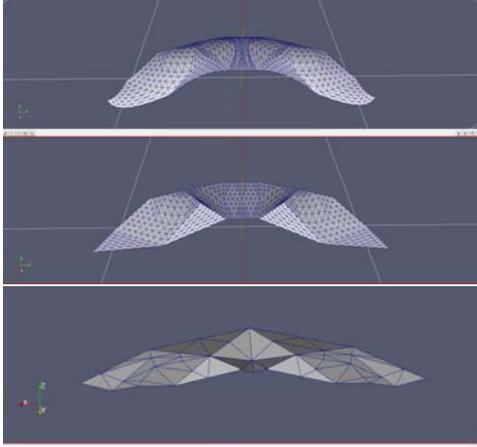
Fig. 2. Preprocessed geometrical models of the wing surface used in the three simulations. Top to bottom: higher-order geometry models (“curved” and “sharp” wings) used in FastAero, and the lower-order “sharp” model used in NekTar.
