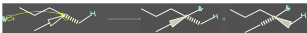
Figure 7: Nucleophilic addition involves a charged electrophile and a nucleophile. The reaction produces a racemic mixture of stereoisomers.
