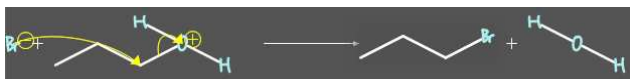
Figure 9: In this concerted nucleophilic substitution process, the leaving group dissociates from the carbon atom while the bromine ion attaches to the backside, resulting in inverted stereochemistry.
