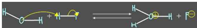
Figure 2: An acid-base reaction between hydrofluoric acid and water. Water, which acts as a base in this situation, removes a proton from the acid to produce a fluorine ion and water's conjugate acid, which is weaker than hydrofluoric acid.
