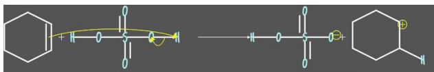
Figure 6: In this electrophilic addition transformation, electrons from a pi-bond attach to an electrophile of a polar solvent (in this case the hydrogen of sulfuric acid).
