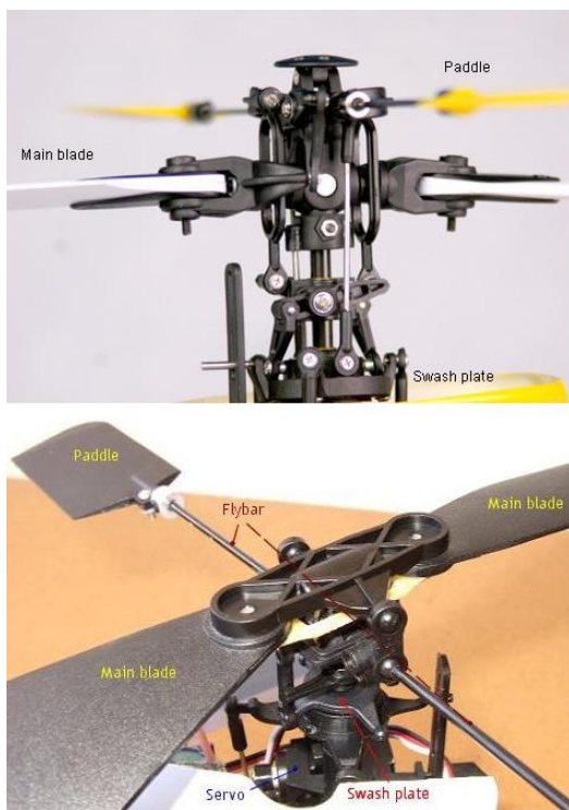
Figure 2: Comparison of Head Assembly (Top, 6-channel; Bottom, 4-channel)
