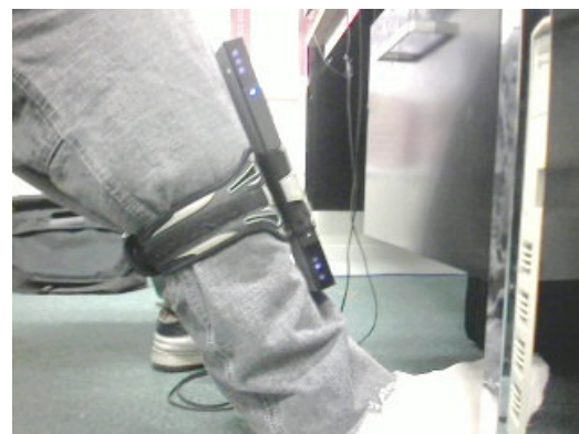
Figure 3: Players were required to wear infrared emitters attached to their legs in order for the wiimote to detect motion and gestures
