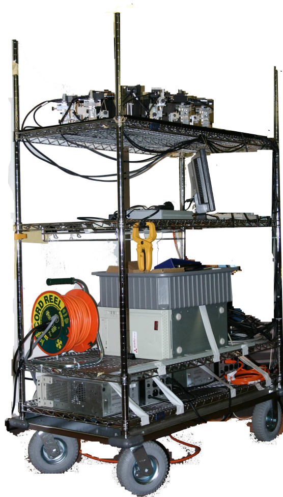
Figure 7.1: The mobile optical workbench with the splitting tree system on top, at eye level.
