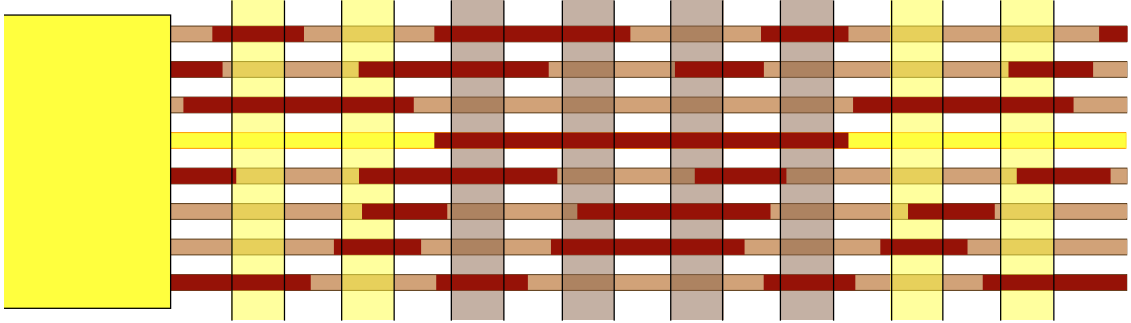
Figure 3.3: An encoded NW decoder in which each NW has a sequence of lightly and heavily doped regions along its axis. When a subset of the MWs is activated, all NWs with lightly doped regions under those MWs become nonconducting. This allows MWs to address NWs with a particular encoding. Since encodings are assigned randomly to NWs, the probability that many NWs are individually addressable is determined by the total number of possible encodings. Fluidic assembly cannot guarantee that lightly doped regions align with MWs.
