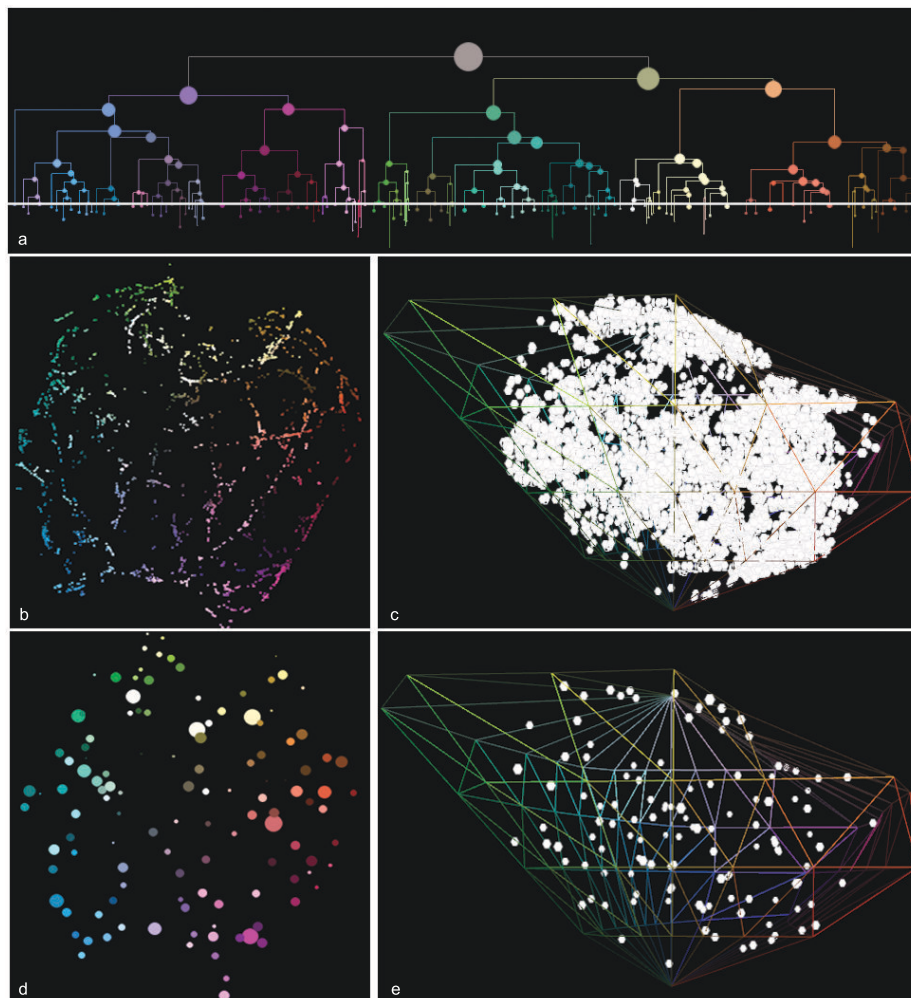
Figure 4.6: A clustering cut in the dendrogram view (top row) is applied to the linked 2D embedding and 3D colorer (middle row). Points belonging to the same cluster are collapsed to their centroids (bottom row).
