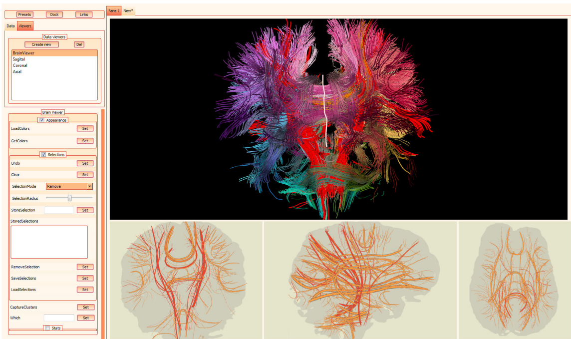
Figure 4.5: An interactive analysis system using linked views and planar tract-bundle projections. Three planar representations, along the coronal, transverse and sagittal planes (bottom panels), are linked to a 3D streamtube model (upper left) and a 2D point embedding of tract similarities (upper right). Selections in the projection views can be performed by clicking or cutting across cluster curves and are mirrored in the 3D view. Points corresponding to the selected tracts are interactively embedded into the plane and used to refine selections at tract level.
