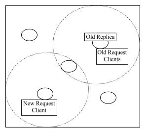
Fig. 2.1: Before applying any algorithm. In this diagram, dotted lines represent latency constraints, and solid line circles represent Tapestry servers.
