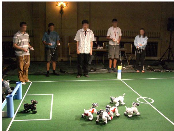
Figure 1: Users controlling Aibos with Wiimotes
