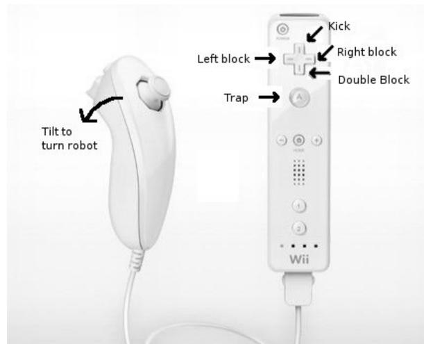
Figure 5: Wiimote control interface for the Aibo
