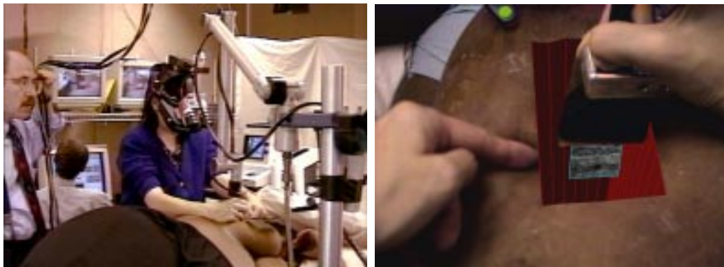
Figure 10: Surgical trial of augmented reality headset used in breast biopsy at the University of North Carolina at Chapel Hill. The surgeon, wearing the video see-through headset (left image) sees simultaneously the patient and the potential tumor inside the patient (right image), displayed by the computer using live, real-time, ultrasound data.
