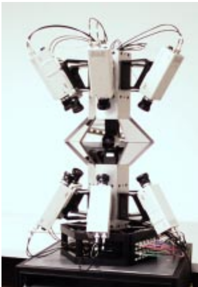
Figure 12: The "Camera Cluster" is an optical device which uses multiple cameras to create a very high resolution, full 360 degree image with a common center of projection. It is especially useful for video conferencing and other applications, such as surround video or movies, where a strong feeling of "presence" is desired. The device was created and developed by UNC's Microelectronic Systems Laboratory in the Computer Science Department and the mechanical structure was designed and built by the University of Utah.
