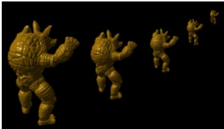
Figure 2: Our appearance-preserving model simplification process reduces the number of polygons needed to display a model while maintaining the visual appearance. The ability to trade precision for rendering speed increases the complexity of the models we can work with.
