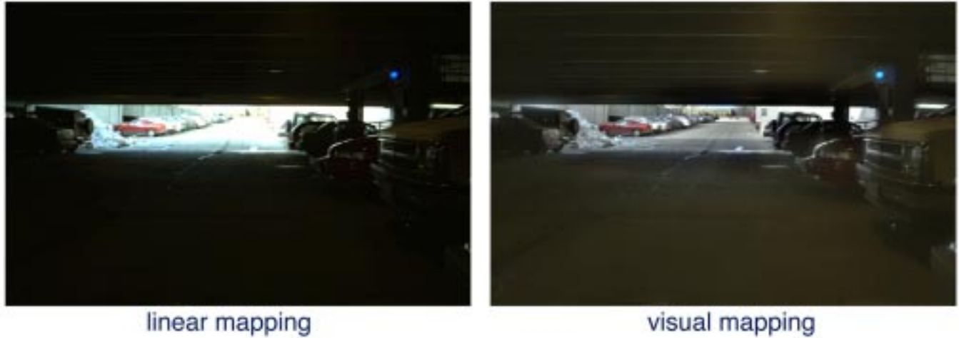
Figure 3: This figure illustrates how the multiscale visual model can be applied to the problem of displaying high dynamic range scenes on low dynamic range devices like CRT's and printers. The scene has a dynamic range of approximately 10,000:1 from highlights to shadows. The printed page has a dynamic range of less than 50:1. A typical linear mapping of the scene luminances produces the image shown on the left, which shows burnout and blackout in the bright and dark regions. Using a mapping based on the multiscale visual model produces the image on the right, which preserves detail across the full range of scene luminances and is much closer to our visual experience of the scene.
