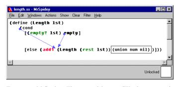
Figure 10. MrSpidey: The static debugger (Windows version).
