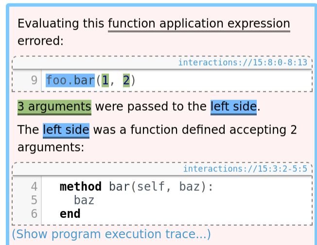
Figure 6. An implicit structure causes an apparently contradictory message: the message references “3 arguments”, but the corresponding highlight selects only two arguments. A ‘self’ parameter has been passed implicitly to the method in the application. The presence of an implicit structure creates an apparent discrepancy between the message text and its corresponding highlight.
